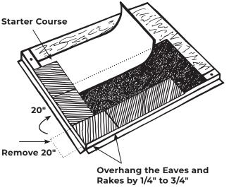
Apply full-length IKO Leading Edge Plus starter strips to the remaining eave and rake edges of the roof deck. Install the starter strips granule side up with the factory applied sealant adjacent to the edges. The starter strips should overhang the rake edge and eaves by 1/4" to 3/4". Fasten the starter strips to the roof deck with nails located 3" to 4" from the eave edge, 4 nails per starter strip.
